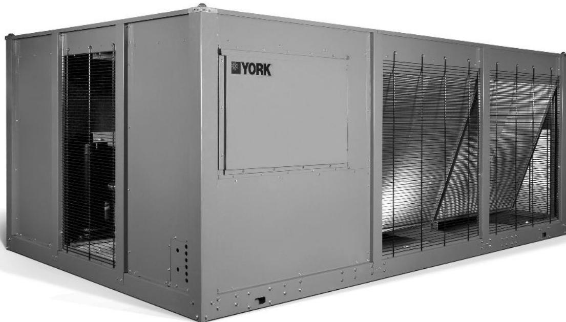
**YORK** Air-Cooled Scroll Chillers provide chilled water for all air conditioning applications using central station air handling or terminal units. They are completely self-contained and are designed for outdoor (roof or ground level) installation. Each unit includes hermetic scroll compressors, a liquid cooler, air cooled condenser, a charge of refrigerant R-410A, and a weather resistant microprocessor control center, all mounted on a rugged, formed-steel base.
