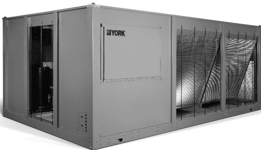
**YORK** Air-Cooled Scroll Chillers provide chilled water for all air conditioning applications using central station air handling or terminal units. They are completely self-contained and are designed for outdoor (roof or ground level) installation. Each unit includes hermetic scroll compressors, a liquid cooler, air cooled condenser, a charge of refrigerant R-410A, and a weather resistant microprocessor control center, all mounted on a pressed-steel base.
