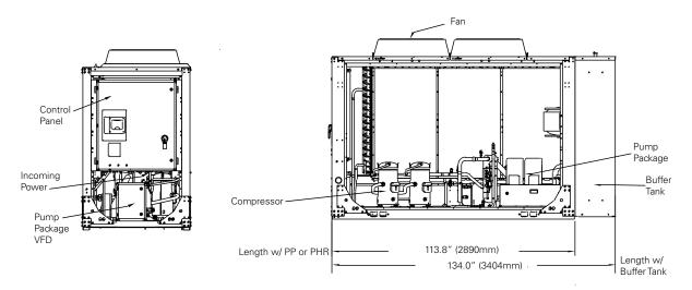
Figure 19. CGAM 30 and 35 ton - pump package, buffer tank, partial heat recovery
