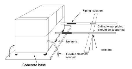
For maximum isolation effect, water lines and electrical conduit should also be isolated. Wall sleeves and rubber isolated piping hangers can be used to reduce the sound transmitted through water piping. To reduce the sound transmitted through electrical conduit, use flexible electrical conduit.
