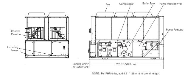
Figure 24. CGAM 130 ton - pump package, buffer tank, partial heat recovery
