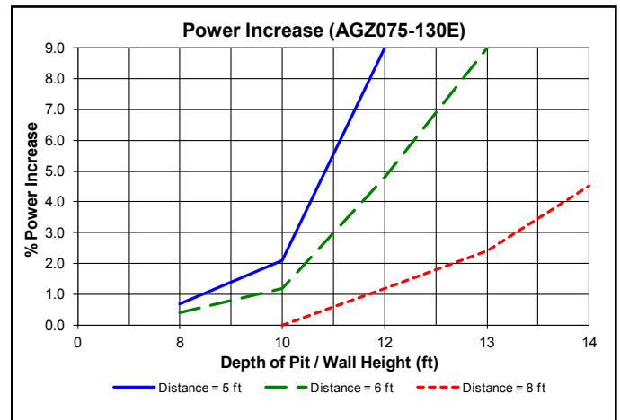
Figure 16: Case 5 - Power Increase (AGZ075-130E)
