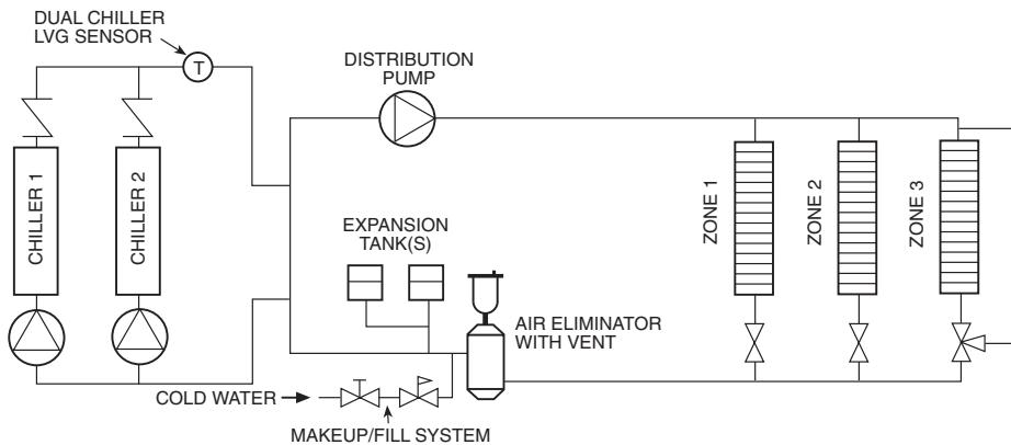
The leaving hot-water temperature is a function of the entering hot water temperature, hot water flow and chiller capacity. In the heat reclaim mode, the entering hot water temperature, and not the leaving hot water temperature, is controlled. As a consequence, these applications are useful for make-up water or preheating of process hot water systems that have alternative means of controlling the desired hot-water temperature.
