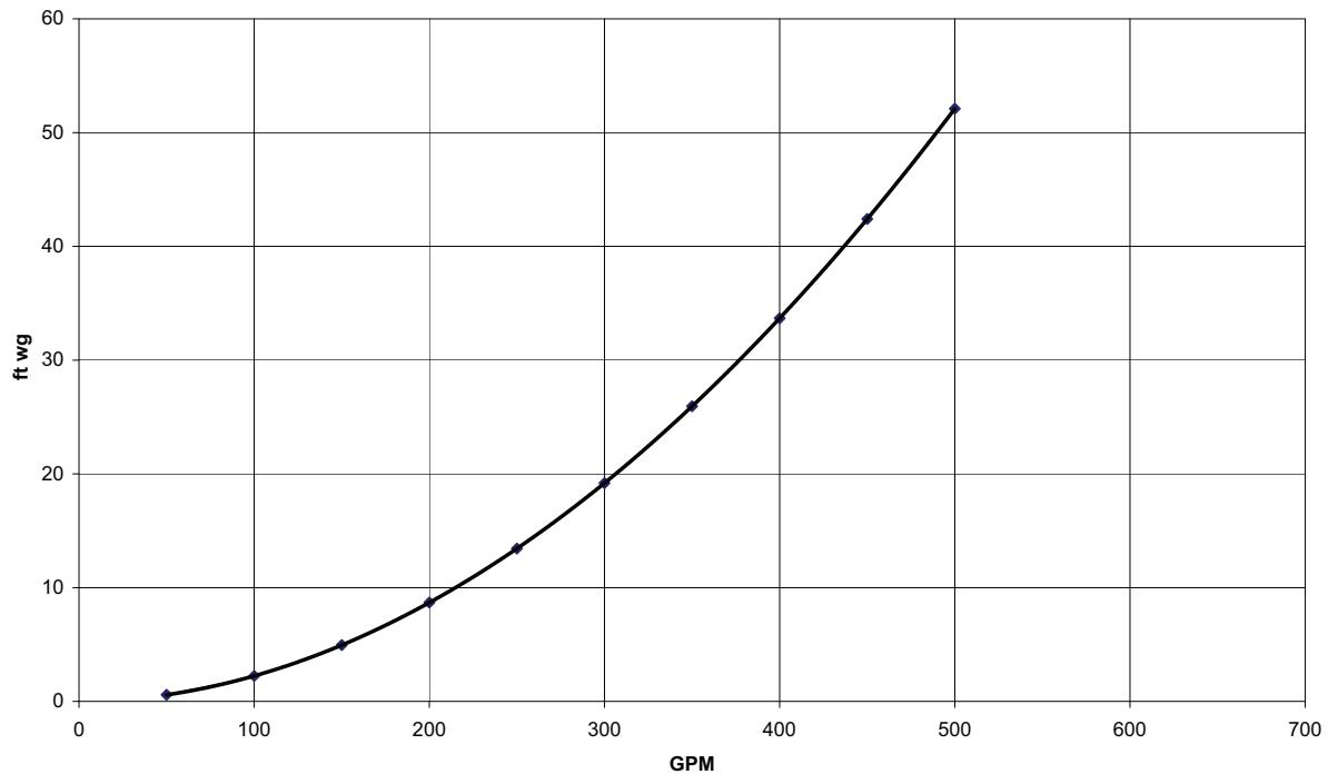
HEAT RECLAIM VESSEL PRESSURE DROP CURVES
