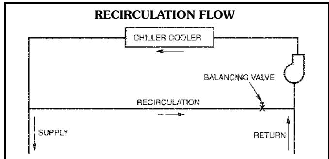
**Maximum cooler flow** — The maximum cooler flow (approximately 5° F [2.8° C] rise) results in a practical maximum pressure drop through cooler.
