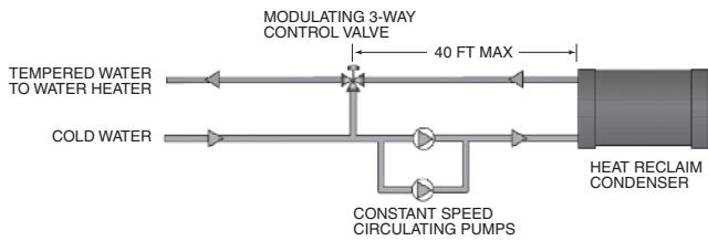
NOTE: Locate the 3-way valve as close as possible to the chiller to minimize head pressure control response time.
